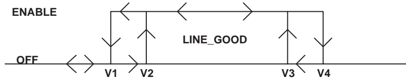
Figure 2. Line UVLO and OVLO Operation
